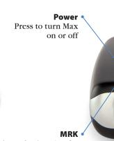
To mark a location for future alerts, press MRK twice, then VOL + or to select the type of marker, then MRK again to confirm. Press twice while receiving marker alert to unmark
