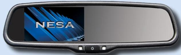
The NSR-43LAD is a replacement mirror with a built in 4.3" LCD monitor with distance guidelines. The screen and mirror are both auto-dimming to automatically adapt to ambient lighting. In normal use the mirror looks standard until the car is placed in reverse and the image appears. 2 inputs allows for multiple cameras or RCA sources to connect. Vehicle specific mounting brackets available.
