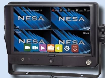
The NSM-90GPS DVR is a quality 9" quad monitor with integrated drive recorder, all operated via a responsive touchscreen and the easy to use operating software. It can connect up to four cameras to record real time video to four Micro SD cards (one per camera) and log the GPS position of the vehicle.
