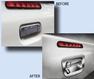
Professional look and sleek design – The Hilux/Ranger tailgate handle surround is so simple to install – just stick on with the included double sided tape and thread the cable through. No need to drill any holes. The end result is factory OEM look. The high quality CCD camera produces a bright clear image. Available in chrome only.
